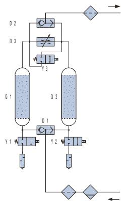
The dryer consists of two drying columns (Q1 and Q2), which alternatively goes into operation or regeneration mode. The cartridge, through which the compressed air passes, dries it and absorbs the water contained in the air. Meanwhile, the second cartridge is flown through in reverse direction by expanded dry air and hence dried out. After some time the two columns are interchanged and the drying process is continued with the column regenerated earlier.
