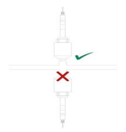
In order to prevent accumulation of condensation in the case of a fault, the device must be vertically screwed onto the line from above.
