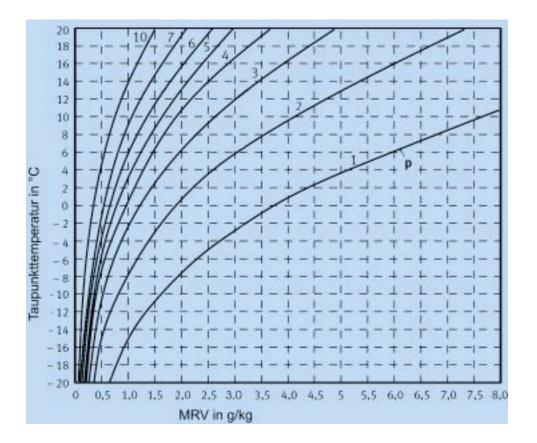
In order to evaluate the absolute humidity content (e.g. MRW) of air, it is therefore often advantageous to measure the dew point in the compressed gas (at higher pressure). Because of the measuring principle of the capacitive polymer sensors used here, exact measured values can be achieved same as measurement in expanded air.
