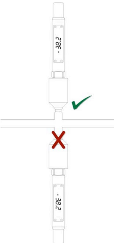
Standing up, long branch lines restrict the response mode or lead to false measured values.
