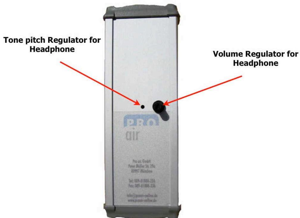
**The enclosed control is insertable and fits for the left notch to adjust the tone pitch, as well as the right notch to adjust the volume.**
