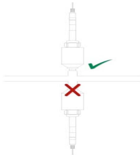
In order to prevent accumulation of condensation in the case of a fault, the device must be vertically screwed onto the line from above.
