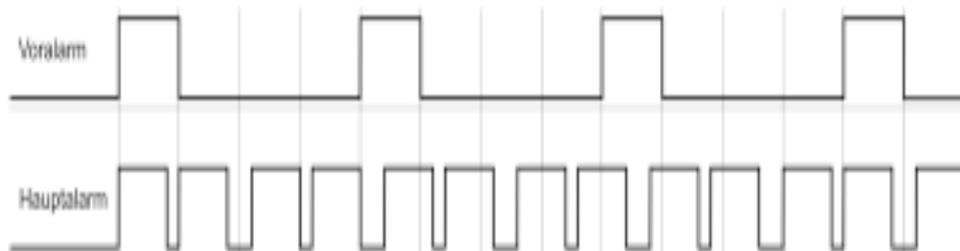
With the Enter key on the keyboard, the acoustic signal can be acknowledged and switched off. However, the optical signal remains still active until the disturbance is removed and the pressure dew point again lies within the alarm limit.
